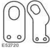
Engine Lifting Brackets 303-1129
